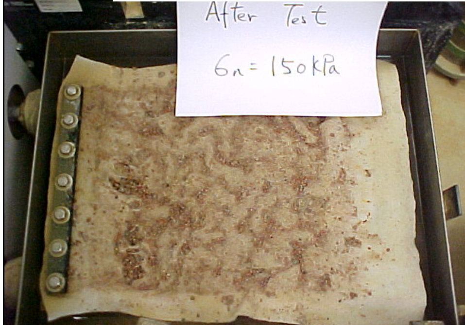
Large direct shear tests on soil-geomembrane interface
