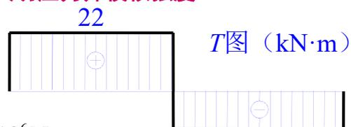
$$\text{AB段 } \tau_{1,\max} = \frac{T_1}{W_{p1}} = \frac{22 \times 10^6 \text{ N}\cdot\text{mm}}{\frac{\pi}{16}(120\text{mm})^3} = 64.8\text{MPa} \quad 14$$
